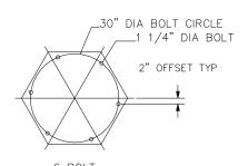
6 BOLT BASE BOLT PATTERN 1 1/4" BASE PLATE THICKNESS AT ANCHOR BOLT VIEW A-A NOT TO SCALE
